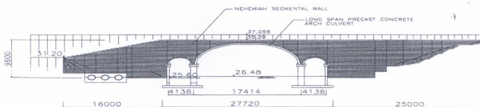
Figure 1: Rear elevation of the segmental wall at Putrajaya
