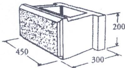
Figure 3: A single hollow-core modular concrete block
