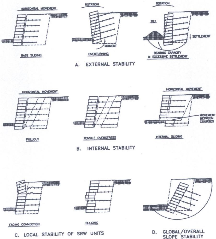
Figure 6: Modes of failure of segmental wall (Simac et al, 1993)
