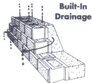
Figure 4: Modular blocks dry stacked together
