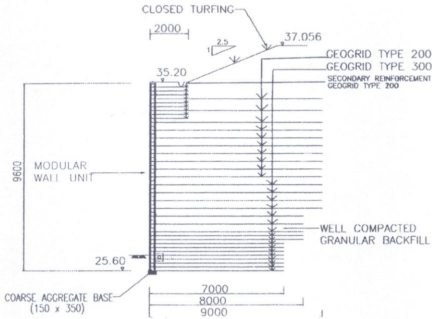
Figure 2: Typical cross section of the 9.6 m high segmental wall
