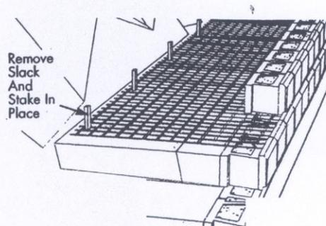
Figure 8: Installation of first layer of geogrid
