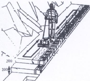
Figure 7: Compaction of backfill
