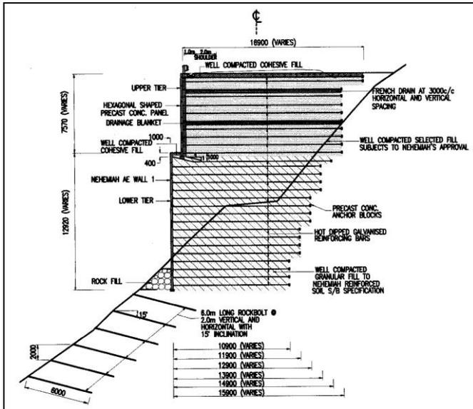
Figure 2: Typical Design Cross Section of Nehemiah Wall
