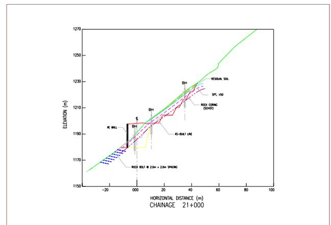
Figure 1: Geological Ground Profile
