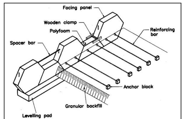
Figure 5: Construction of AE Wall
