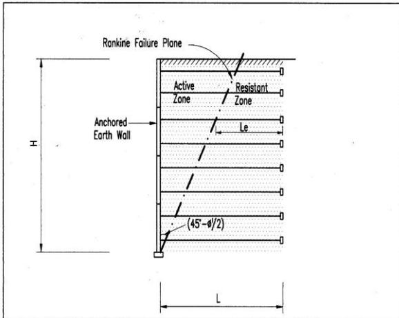
Figure 4: Effective Length of Reinforcing Tendons -  $L_e$
